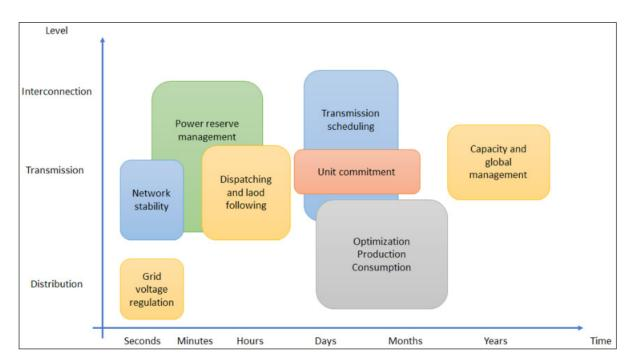
Figure 1. Different applications use forecasting data with different time intervals [8].
