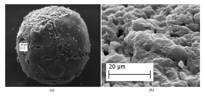
Figure 3. SEM micrographs of the m-poly(DVB-VIM) microbeads in (a) and (b).
