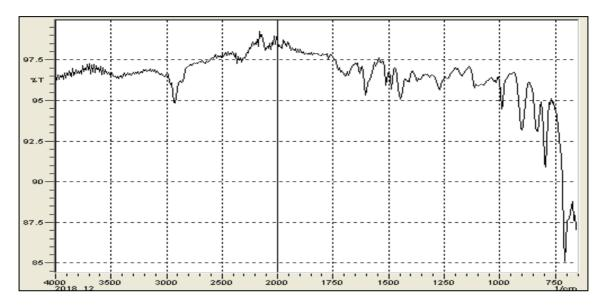
Figure 2. FTIR results of m-poly(DVB-VIM) microbeads.
