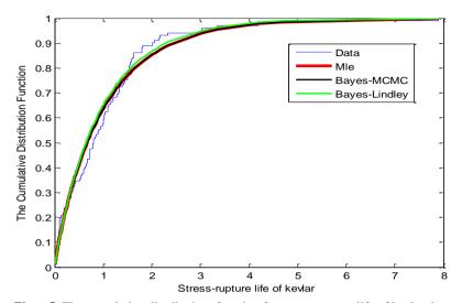
Figue 5. The cumulative distribution function for stress-rupture life of kevlar data
