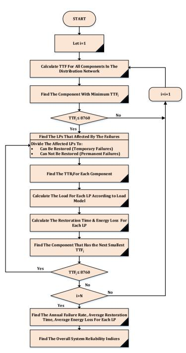
Figure 7. Flowchart for evaluation reliability of distribution system based on MCS
