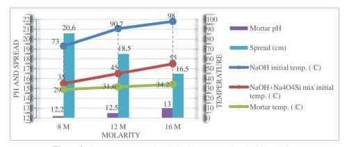
Figure 2. Temperature, spread and pH changes associated with molarity
