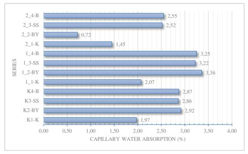
Figure 8. Capillary water absorption percentage of 2nd series geopolymer mortars
