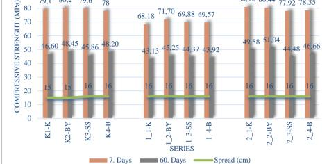
Figure 7. Compressive strength and spread values of 2nd series geopolymer mortars
