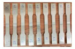
Figure 2. Test specimens prepared according to EN ISO 6892-1 Standard
