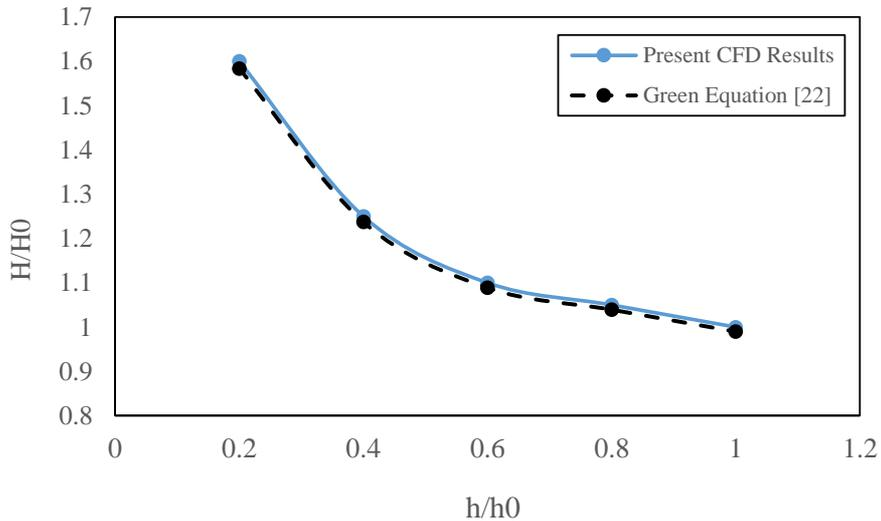
**Figure 3.** Comparison of results of present numerical work and theory [22] for dimensionless variation in wave height vs. depth in the model with a 30° oblique left-side oscillating wall
