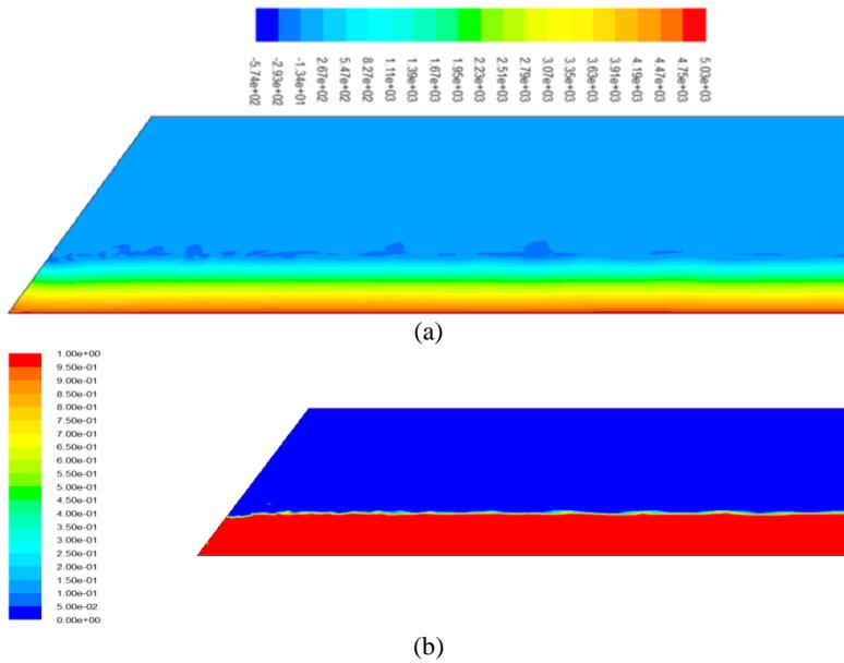
**Figure 9.** a) Pressure contour b) Vorticity contour (changes in tank water level) for a tank with a 30° oblique left-side oscillating wall at  $t=0.5$ s
