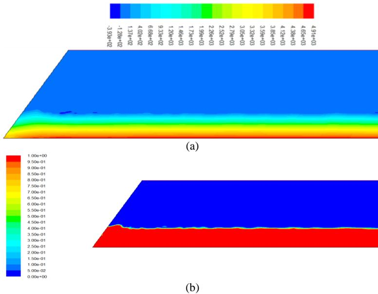
**Figure 10.** a) Pressure contour b) Vorticity contour (changes in tank water level) for a tank with a 30° oblique left-side oscillating wall at  $t=1.0$ s
