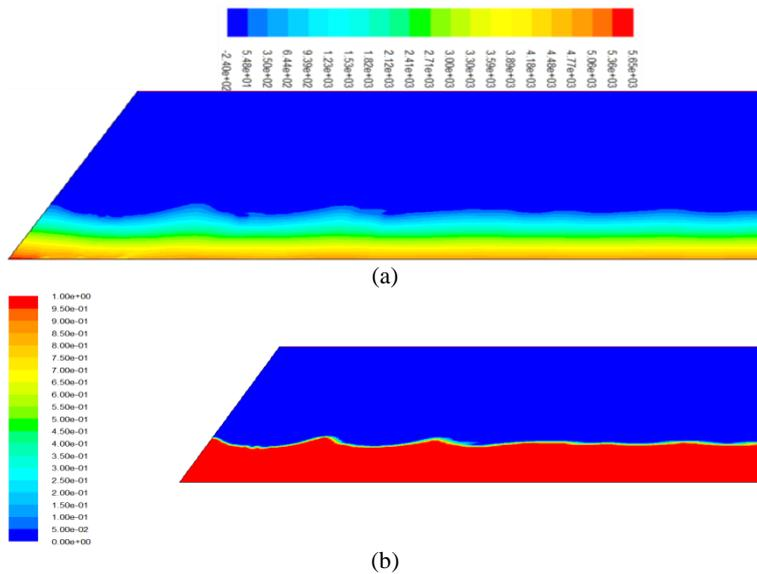
**Figure 13.** a) Pressure contour b) Vorticity contour (changes in tank water level) for a tank with a  $30^\circ$  oblique left-side oscillating wall at  $t=4.0s$
