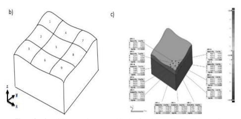
Figure 3. After milling operations. a) Machined surface b) 9 equal area c) 3D scan view
