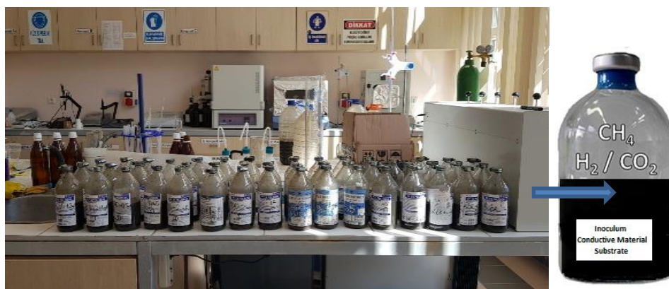
Figure 1. Anaerobic batch digesters
