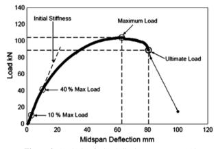
Figure 3. Analysis of a load-displacement curve [12].
