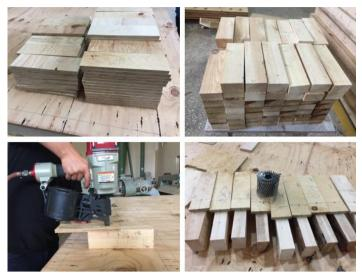
Figure 1. Preparation of specimens for lateral nail strength test
