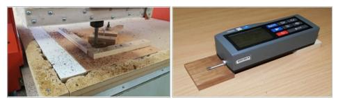
**Figure 3.** CNC machine (*BDARK 2120 PRO, Turkey*) in face milling operation
