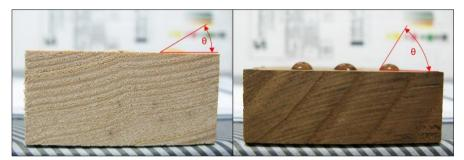
**Figure 2.** Contact angle measurement  $(\theta)$  on untreated and thermo-treated ash wood samples
