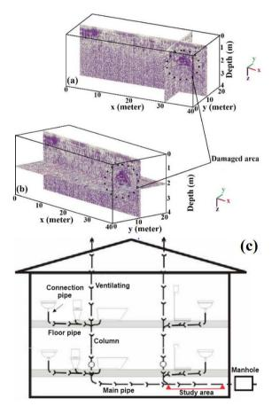
**Figure 4. a)** 3D image of damaged area by intersection of *X* and *Y* sections, **b)** Slice image of damaged area by intersection of *Y* section, **c)** Indoor wastewater installation pipe sections and representative study area (designed from URL-1, 2018).
