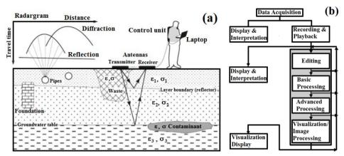
Figure 2. a) Representation of main components and principle of GPR system (modified from Knödel *et al.* [2]), b) Data processing stages of GPR method (modified from Annan [28]).
