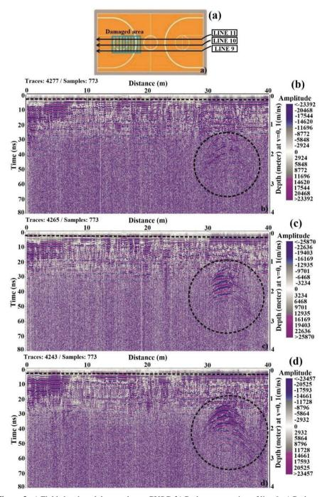
**Figure 3. a**) Field sketch and damaged area GUSC, **b**) Radargram section of line 9, **c**) Radargram section of line 10 and, **d**) Radargram section of line 11.
