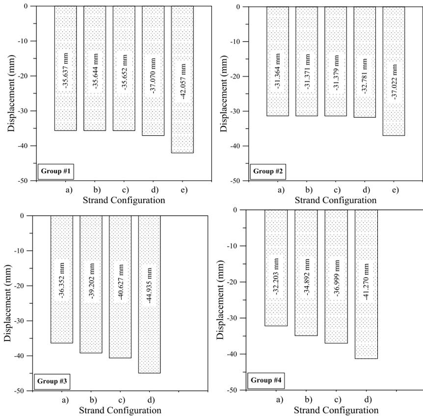
Figure 13. The maximum displacements of girders at mid-span
