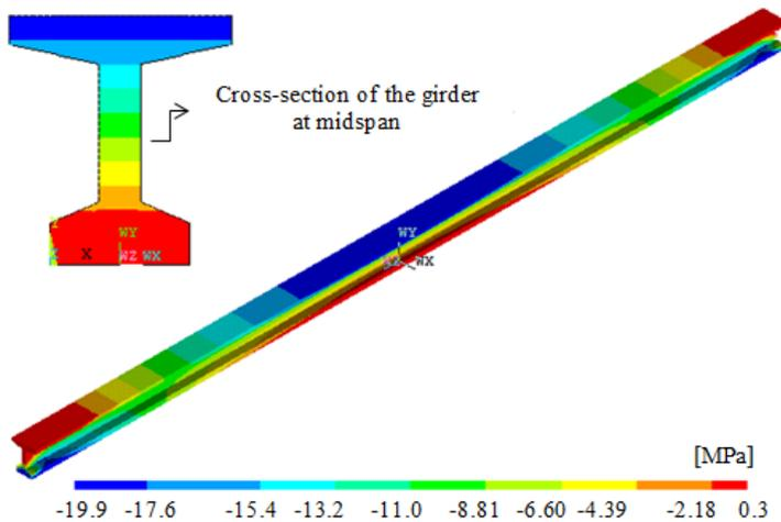
Figure 10. The maximum principal stress contour for girder (a) in Group #1
