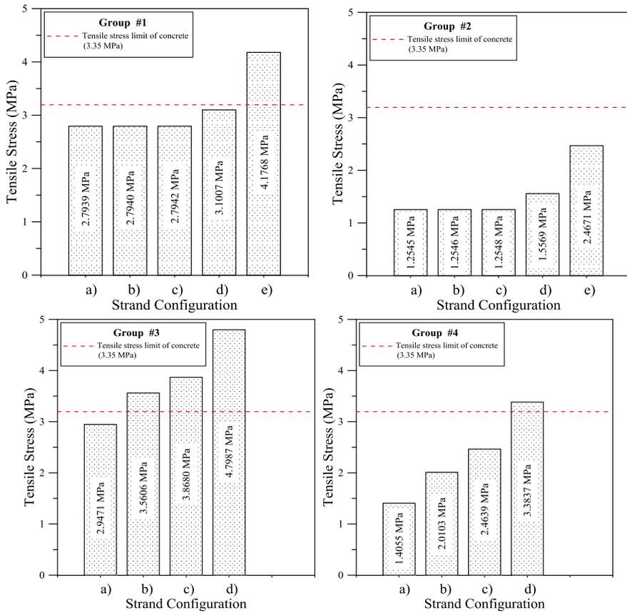
Figure 9. The maximum tensile stresses of girders at mid-span.
