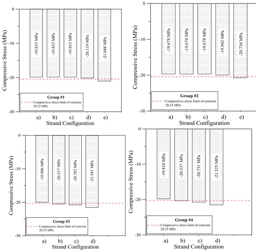
**Figure 11.** The maximum compressive stress of girders at mid-span
