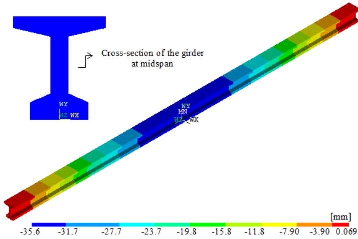
Figure 12. The maximum displacement contour of the girder (a) in Group #1
