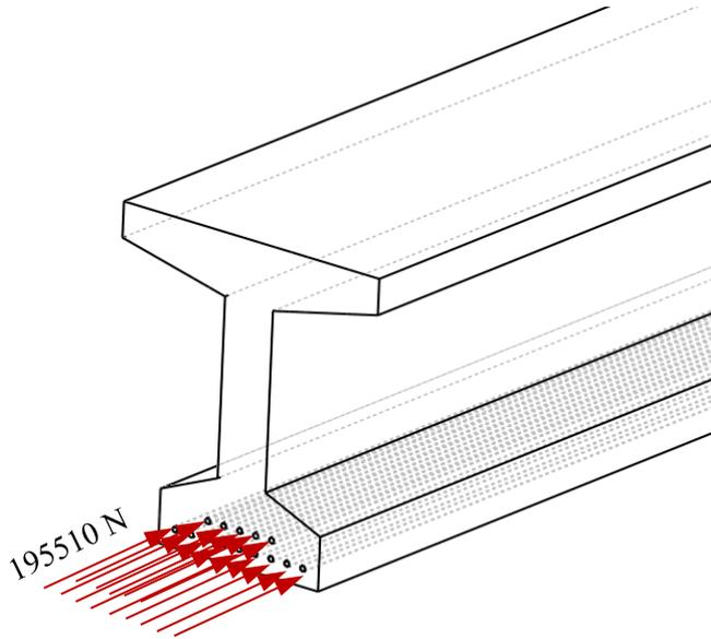
**Figure 7.** Prestressing force for each strand in the girder
