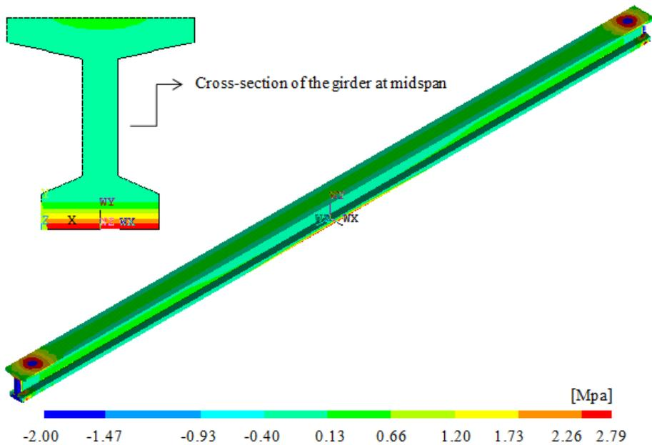
**Figure 8.** The minimum principal stress contour for girder (a) in Group #1
