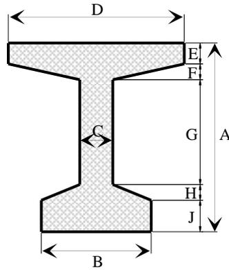
**Figure 1.** Cross-section of the investigated girder
