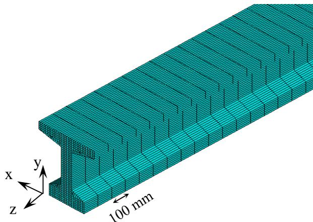
**Figure 6.** Finite element model of the girder
