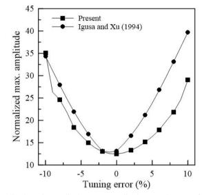
Figure 9. Normalized maximum displacement amplitude vs. tuning error for damped main system with TMD-20 system
