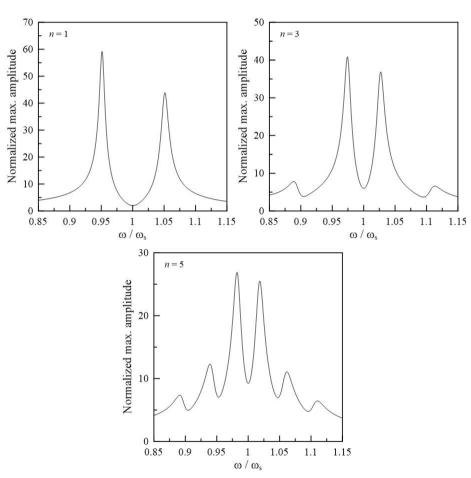
Figure 2. Variation of response amplitude under harmonic excitation for different number of TMD units
