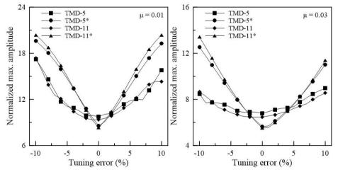
Figure 7. Normalized maximum displacement amplitude vs. tuning error for damped primary system with different MTMDs
