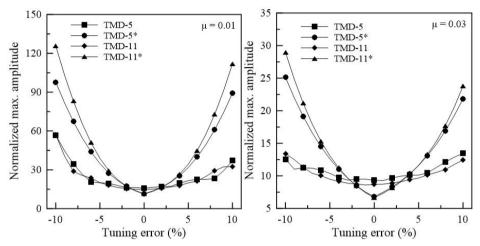
Figure 6. Normalized maximum displacement amplitude vs. tuning error for undamped primary system with different MTMDs
