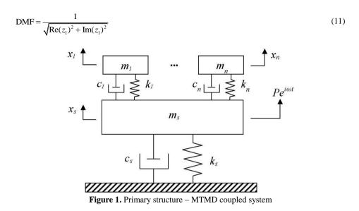
where  $\beta = \omega / \omega_s$  is the frequency ratio between the external force and the structure,  $\xi_s$  is the damping ratio of the structure,  $\mu_j = m_j / m_s$  is the mass ratio,  $\beta_j = \omega_j / \omega_s$  is the frequency ratio, and  $\xi_i = c_i / 2m_i\omega_j$  is the damping ratio of *j*th TMD.
