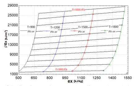
Figure 7. The effects of pressure and temperature on the specific exergy and exergy density of air
