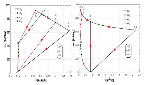
Figure 8. Specific exergy diagrams via the specific entropy and specific volume for air standard power cycles
