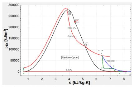
Figure 4. Exergy density and specific entropy diagram for the case thermal power plant
