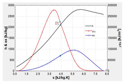
Figure 1. Specific enthalpy, specific exergy, exergy density and specific entropy diagram for water
