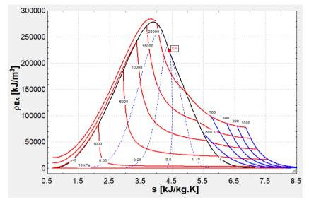
Figure 3. Exergy density and specific entropy diagram for water
