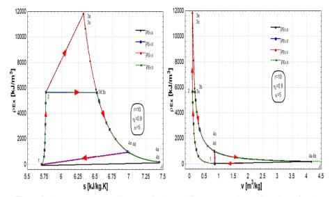
Figure 9. The exergy density diagrams via the specific entropy and specific volume for air standard power cycles
