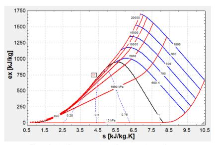
Figure 2. Specific exergy and specific entropy diagram for water
