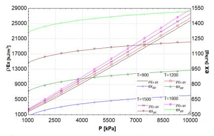
Figure 5. The effects of pressure and temperature on the specific exergy and exergy density of air
