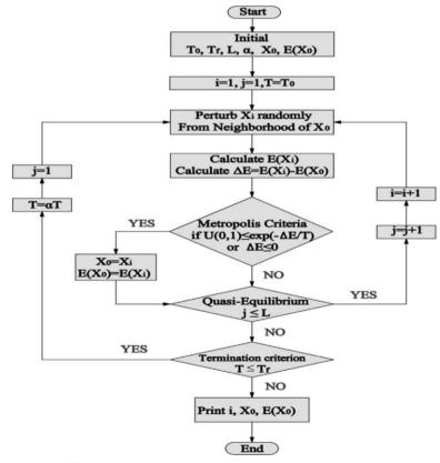
Figure 1. Flowchart of the simulated annealing algorithm.
