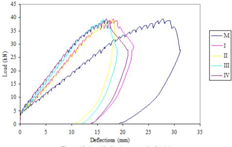
Figure 13. Load Deflection curve of AG4 slab
