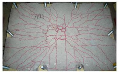
Figure 16. Failure pattern of AGD4 slab
