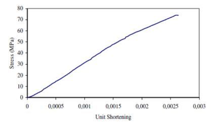
Figure 1. Stress-Strain curve for high-strength concrete
