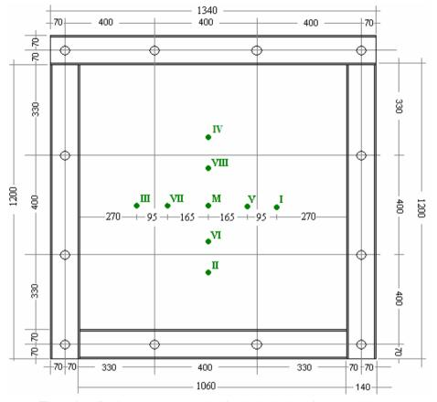
Figure 6. Deflection measurement points for 1060x1060 mm free-span slabs [16]
