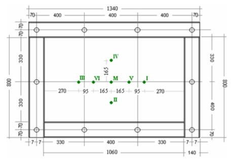
Figure 5. Deflection measurement points for 660x1060 mm free-span slabs [16]
