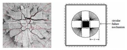
Figure 19. Experimental and theoretical failure mechanisms of a fixed boundary slab
