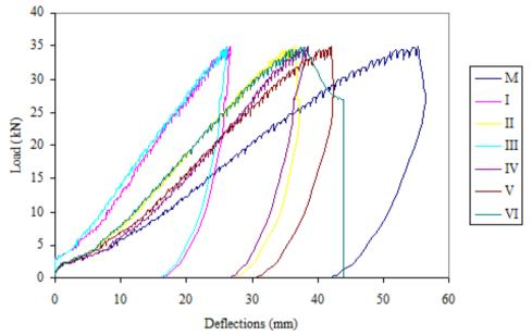
Figure 15. Load Deflection curve of AGD4 slab
