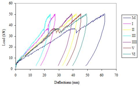
Figure 9. Load Deflection curve of AD4 slab
