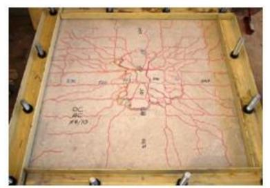
Figure 18. Failure pattern of AGB4 slab
