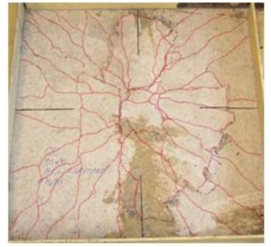
Figure 14. Failure pattern of AG4 slab
