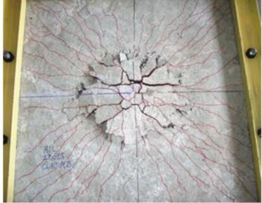
Figure 12. Failure pattern of AB4 slab
