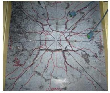
Figure 8. Failure pattern of A4 slab
