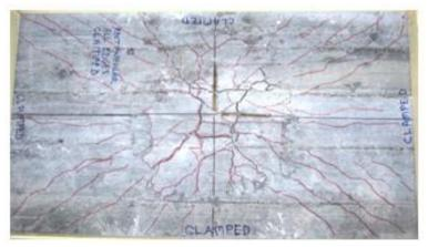
Figure 10. Failure pattern of AD4 slab
