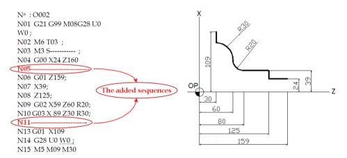
Figure 10. Example of a machining program
