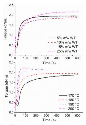
Figure 5. Torque graphs of Silicone/Waste Tyre composites
