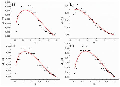
**Figure 6.** Experimental and fitted data for Silicone/Waste Tyre at (a) 170 °C (b) 180 °C (c) 190 °C (d) 200 °C (Black dot: Experimental data; Red curve: Fitted data)
