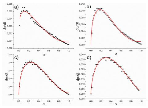
**Figure 2.** Experimental and fitted data for EPDM/Waste Tyre at (a) 170 °C (b) 180 °C (c) 190 °C (d) 200 °C (Black dot: Experimental data; Red curve: Fitted data)
