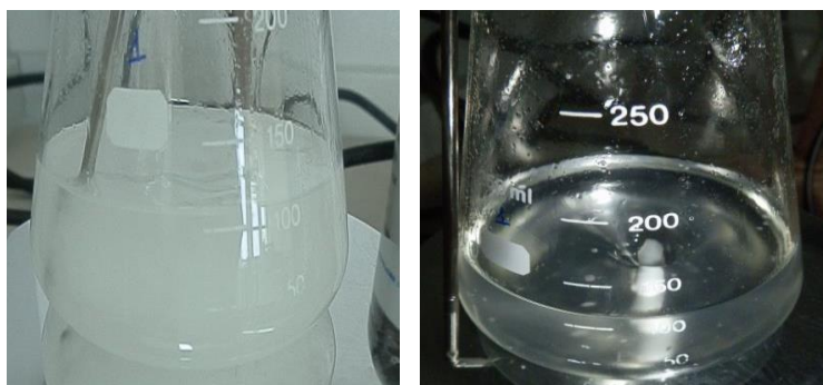
Figure 4. a. Cellulose in the beginning of acetylation reactions and b. clear acetylation system after completed acetylation reactions.
