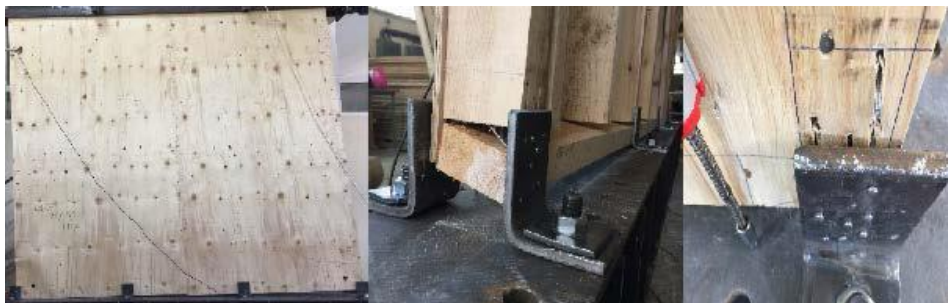
Figure 6. Deformations at the end of the experiment in the shear wall sheathed 5-ply spruce plywood
