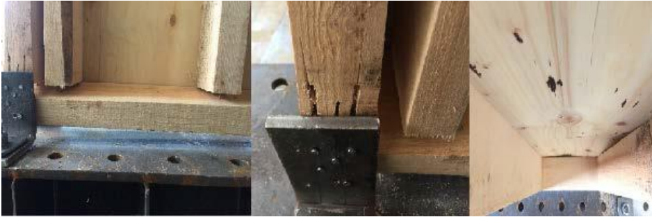
Figure 7. Deformations at the end of the experiment in the shear wall sheathed 7-ply spruce plywood
