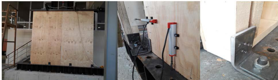
Figure 5. Deformations at the end of the experiment in the shear wall sheathed 7-ply Scots pine plywood
