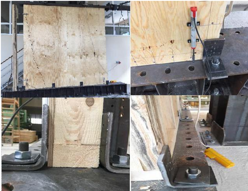
Figure 2. Mounting of shear wall to floor
