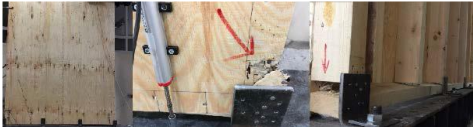
Figure 4. Deformations at the end of the experiment in the shear wall sheathed 5-ply Scots pine plywood
