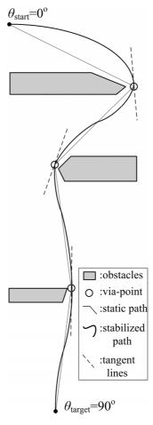
Figure 4. Obstacle free stabilized path by EEDT and MPC
