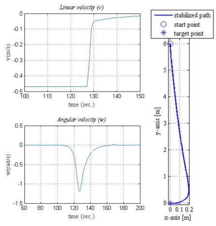
Figure 5. Input control signals and the stabilized path
