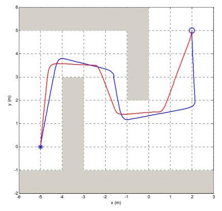
Figure 7. Planned trajectories with state-bounding and MPC-EEDT approaches
