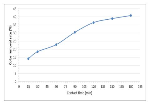
Figure 3. Effect of contact time on color removal efficiency for WMH
