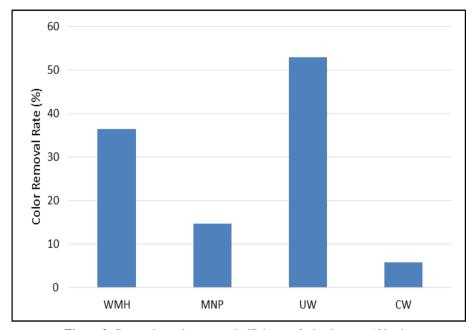
Figure 2. Comparing color removal efficiency of adsorbents at 120 min.
