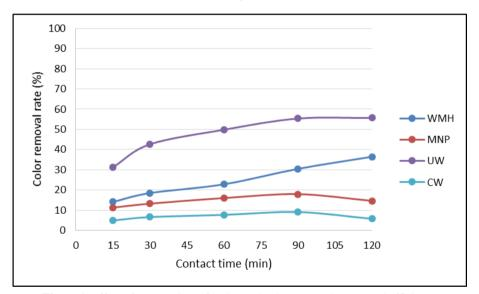
Figure 1. Effect of contact time of various adsorbents on color removal efficiency
