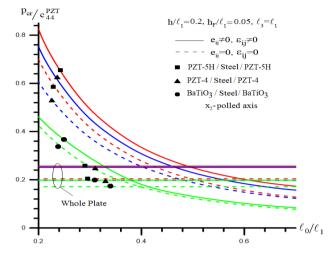
**Figure 4.** The critical buckling delamination force values of the PZT/Steel/PZT sandwich rectangular thick plate for the different PZT materials and  $\ell_0$  crack lengths
