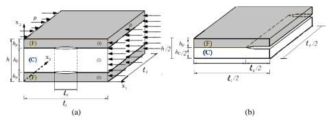
Figure 1. The geometry of the plate and the considered external forces; solution domain (a), oneeighth of the region (b)
