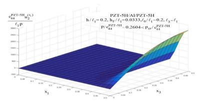
**Figure 2.** The surface graph of the PZT-5H/Aluminum/PZT-5H sandwich rectangular thick plate for  $p / c_{44}^{PZT-5H} = 0.2604$  in the section  $x_2 = h_F + h_C + 0^+$
