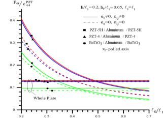
Figure 3. The critical buckling delamination force values of the PZT/Aluminum/PZT sandwich rectangular thick plate for the different PZT materials and  $\ell_0$  crack lengths
