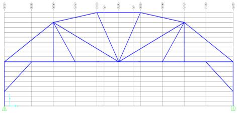
Figure 5. FE model of the steel bridge
