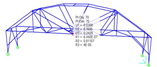
Figure 6. Displacement values in FE model
