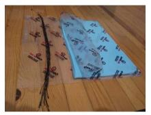
Figure 6. Silicone rubber paste and reinforcing fibers
