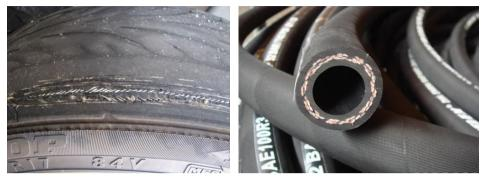
Figure 1. Examples of various fiber-reinforced rubbers [9-10]
