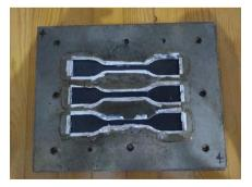
Figure 5. Specimen preparation die
