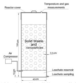
Figure 1. Schematic view of the aerobic bioreactors used in the study
