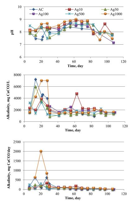
Figure 2. Variations of pH and alkalinity values of leachate in all bioreactors
