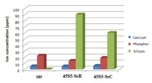
Figure 3. The changes in calcium, phosphor and silicon concentrations of SBF solution with the strontium substituted bioactive glass immersion on 28th day
