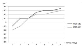
Figure 5. The pH variation of TRIS solution with soaking time for 45S5-SrR and 45S5-SrC sample
