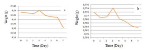
Figure 4. Weight loss of bioactive glass samples in TRIS solution a) 45S5-SrR b) 45S5-SrC
