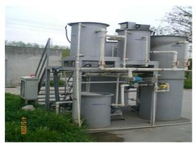
Figure 5.MBR Prototype Facility General Appearance
