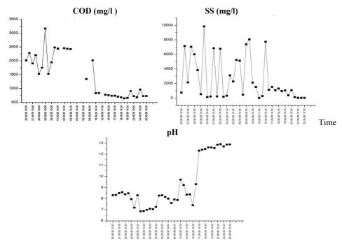
Figure 3. Biological-chemical treatment prototype facility performance graphs
