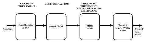
Figure 4. Membrane Bioreactor Prototype Facility flow chart
