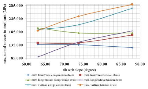
Figure 12. Variation of max. stresses in steel parts depending on slope of rib web.
