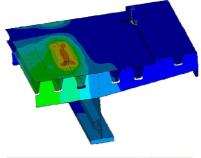
Figure 5. Distribution of deformation vector sum for rib web slope of 73.78°. Max. value is 1.729 mm.
