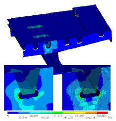
Figure 9. Distribution of von Mises stress with averaged nodal values (top and bottom left) and non- averaged elemet results (bottom right) for rib web slopeof 73.78°. Max. values developed in deck plate, ribs and cross beams are 126.652 MPa, 255.259 MPa and 201.549 MPa
