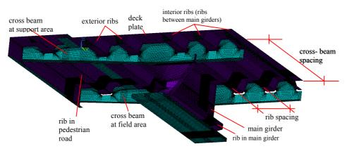
Figure 2. FE- model of orthotropic steel bridge.
