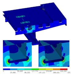
Figure 8. Distribution of von Mises stress with averaged nodal values (top and bottom left) and non- averaged elemet results (bottom right) for rib web slope of 87.92°. Max. values developed in deck plate, ribs and cross beams are 121.538 MPa, 262.34 MPa and 263.612 MPa
