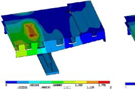
**Figure 4.** Distribution of deformation vector sum for rib web slope of  $87.92^{\circ}$ . Max. value is 1.898 mm.
