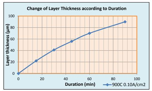
**Figure 4.** The curve indicating the effect of the duration on the thickness of the diffusion layer. The temperature was 900 °C and the current density was 0.10 A/cm<sup>2</sup>
