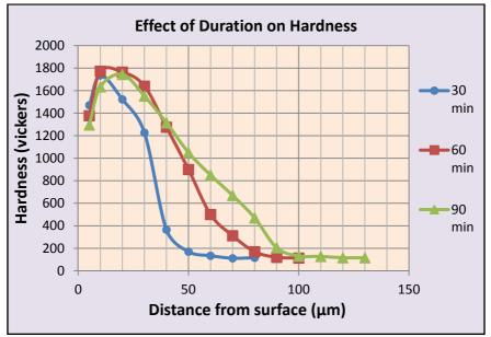
**Figure 9.** Hardness variation as a function of duration for IF steel boronized at 900 °C by applying a current density of 0.10 A/cm<sup>2</sup>
