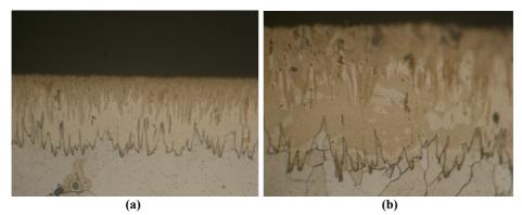
**Figure 5.** Cross-section micrograph of IF steel boronized at (a) 900 and (b) 1020 °C for 45 min by applying a current density of 0.20 A/cm<sup>2</sup> (Scale: 20 μm, Magnification: X500)
