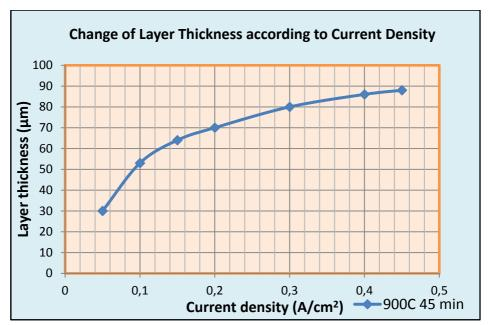
Figure 3. The curve indicating the effect of the current density on the thickness of the diffusion layer. The temperature was 900 °C and the duration was 45 min
