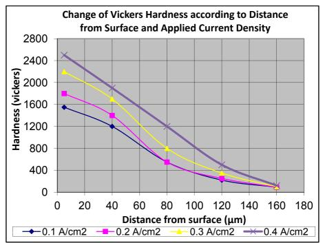
Figure 8. Hardness variation as a function of the applied current densities for IF steel boronized at 900 °C for 45 min
