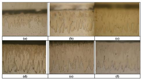
**Figure 1.** Cross-section micrographs of IF steel boronized at 900 °C for 45 min by applying current densities of (a) 0.05, (b) 0.10, (c) 0.15, (d) 0.20, (e) 0.30 and (f) 0.40 A/cm<sup>2</sup>, respectively (Scale: 10 μm, Magnification: X1000)
