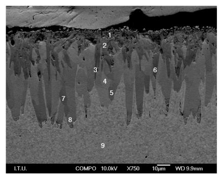
**Figure 6.** SEM micrograph of the IF steel sample boronized at 900 °C for 45 min by applying a 0.10 A/cm<sup>2</sup> density electric current. The marked numbers indicate the points from which EDS analyses were taken
