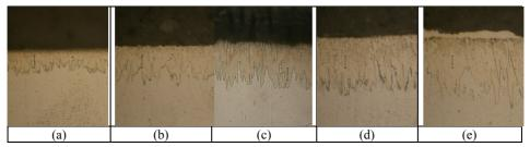
**Figure 2.** Cross-section micrographs of IF steel boronized at 900 °C by applying current densities of 0.10 A/cm<sup>2</sup> for durations of (a) 15, (b) 30, (c) 45, (d) 60 and (e) 90 min, respectively (Scale: 20 μm, Magnification: X500)
