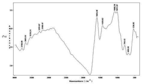
Figure 2c. FT.i.r. spectra of Tunçbilek lignite which oxidized by H<sub>2</sub>O<sub>2</sub> solution
