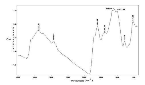
Figure 1b. FT.i.r. spectra of Seyitömer lignite which oxidized by air
