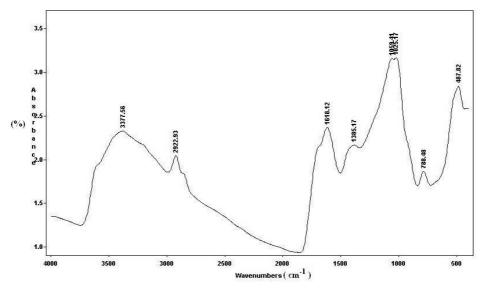
Figure 1c. FT.i.r. spectra of Seyitömer lignite which oxidized by H<sub>2</sub>O<sub>2</sub> solution
