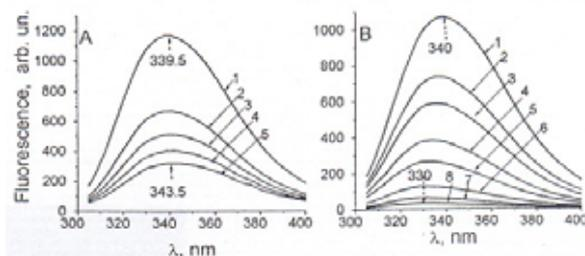
**Figure 94.** Fluorescence spectra of pure BSA (A) and BSA in mixtures of PE + BSA ( $[\text{P50}]/[\text{BSA}] = 3.52$ ) (B) at different concentrations of Cu(II) ions in solution. BSA concentration was 0.71 mg/mL, phosphate buffer (pH 7).  $\text{CuSO}_4$  concentration (in mM): 1, 0; 2, 0.15; 3, 0.3; 4, 0.45; 5, 0.6; 6, 0.9; 7, 1.2; 8, 1.5.
