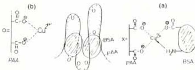
**Figure 102.** A schematic presentation of the formation of chelate units between the functional groups of the PAA and the protein globules with participation of copper ions (b) and structure of ternary PAA-Cu<sup>2+</sup>-protein polycomplexes (a).
