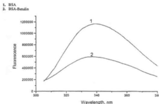
**Figure 169.** Fluorescence spectra of pure BSA (1) and the product obtained from the BSA+betulin+carbodiimide mixture (2), prepared in phosphate buffer (pH 7), BSA concentration in both solution were 0.71 mg/ml
