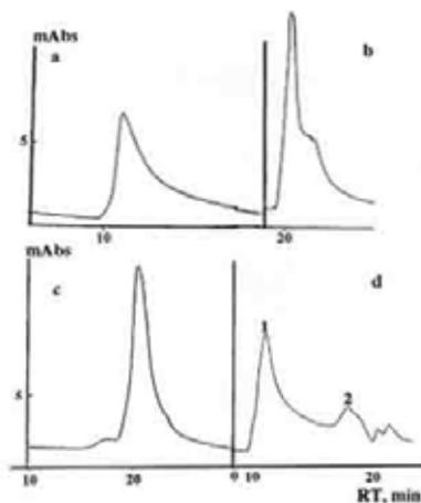
**Figure 175.** Gel filtration HPLC chromatograms of free CP (a), P2 (b), reaction products of CP2-P2 prepared in HRM systems (c) and mixture CP2-P2 (d). RT-retention times, UV-280 nm  $C_{P2} = 2\text{mg/ml}$ ;  $40\mu\text{l}$ . Concentrations of CP2, conjugate and P2:  $3\text{mg/ml}$ ;  $40\mu\text{l}$  injection,  $1\text{ml/min}$ ;  $25^\circ\text{C}$
