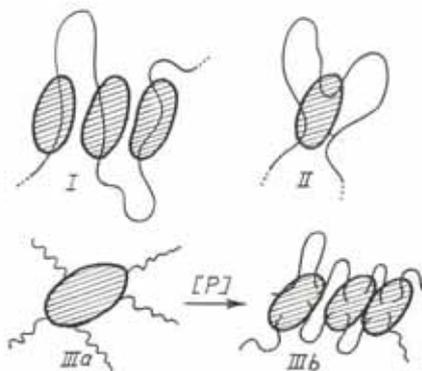
**Figure 130B.** A schematic presentation of the structure of covalent conjugates (PAA-BSA) at different lengths of the polymeric chain (degree of polymerization,  $n$ : 1140 (I), 550 (II) and 43 (III)). At  $n=43$  two types of structures were formed depending on the BSA/PAA ratio. For explanations see text
