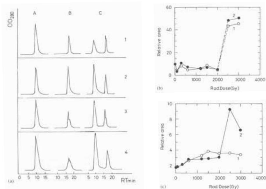
**Figure 190.** (a) HPLC chromatograms of unirradiated and irradiated solutions of PAA (A), SOD (B), PAA + SOD (C); 1 - unirradiated solutions; irradiated solutions at different irradiation dose (Gy): 600 (2); 2500 (3); 3000 (4);  $C_{BSA} = C_{PAA} = 0.01$  g/l (b) Relative area of the peaks, corresponding free PAA (1) and PAA in mixture PAA-SOD versus radiation dose (2). (c) Relative area of the peaks, corresponding free SOD (1) and SOD in mixture PAA-SOD versus radiation dose (2)
