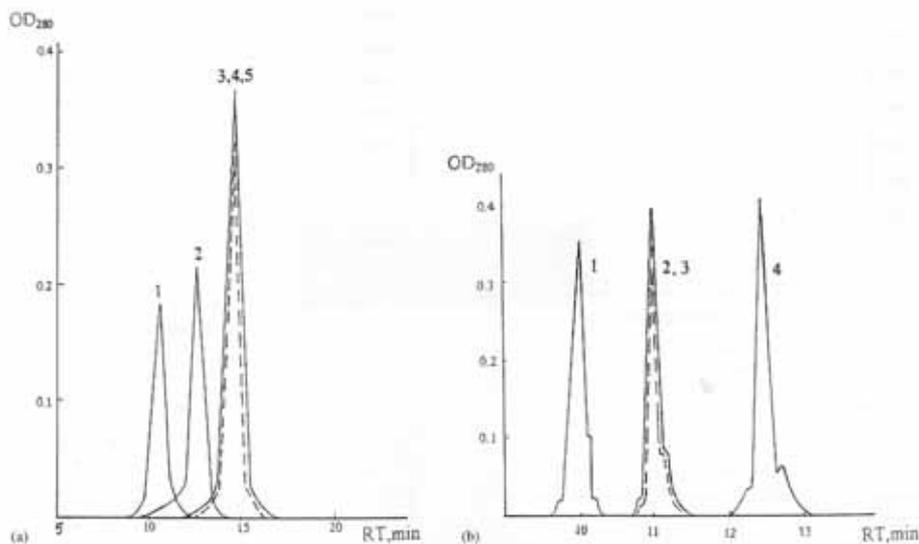
**Figure 109.** Electrophoregrams of BSA and reaction products of CP-EDC-BSA mixtures obtained at different BSA/CP ratios by two methods: native (a) and SDS-polyacrylamide gel electrophoresis (b). BSA/CP: 0.28 (1); 0.59 (2); 1.14 (3); 1.70. (4); free BSA (5 - native, 4 - SDS). Different polymer concentrations, RT - retention time. Diagrams represent normalized OD<sub>280</sub> values.
