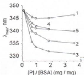
**Figure 99.** Fluorescence parameter  $\lambda_{\text{max}}$  for P + BSA mixtures at the presence of Cu(II) ions (1.2 mM) vs. ratio [P]/[BSA] (phosphate buffer, pH 7). P is polymer with percent of polar residues: 1, 0 (P0); 2, 25 (P25); 3, 50 (P50); 4, (P75); 5, 100 (P100).
