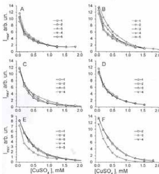
**Figure 96.** Intensity of BSA fluorescence in maxima for a mixture P + Cu(II) + BSA vs. Cu(II) concentration in solution (phosphate buffer, pH 7) at different polymers: A, O (PO); B, 25 (P25); C, 50 (P50); D, 75 (P75); E, 100 (P100); F, the same as E but at pH 5. BSA concentration was 0.71 mg/mL,  $[\text{P}]/[\text{BSA}]$  (mg/mg): 1, 0.58; 2, 0.85; 3, 1.76; 4, 3.52.
