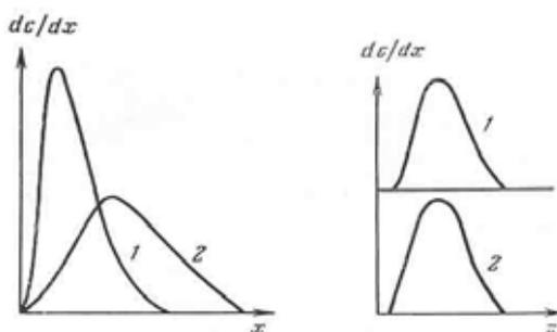
**Figure 105.** Sedimentograms of mixtures BSA-Cu(II)-PVPI (1) and BSA-Cu(II)-PVPII (2) at  $n_{BSA}/n_{PVP}=4(1),10(2); P_w=10^3$  (PVPI) and  $7.4 \times 10^3$  (PVPII)  $t=12$  min.  $\omega=26000$   $\text{min}^{-1}$ . Right sedimentograms corresponds to BSA(1) and BSA-Cu(II) (2),  $t=60$  min.  $\omega=56000$   $\text{min}^{-1}$
