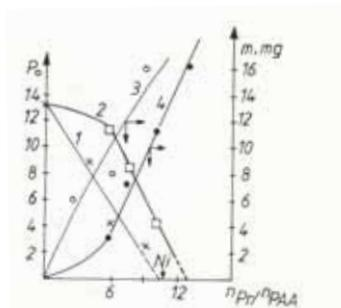
**Figure 85.** Dependence of the chromatogram peak area ( $P_o$ ) of free PMC and the amount ( $m$ ) of the precipitation in Hb-Cu<sup>2+</sup>-PAA (1,3) and GI-Cu<sup>2+</sup>-PAA (2,4) on  $n_{pr}/n_{pAA}$ ;  $C_{PAA} = 0.1$  g/dL;  $n_{Cu}/n_{AA} = 0.08$ ; pH 7.
