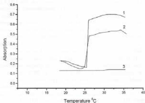
**Figure 113.** Temperature dependence of OD<sub>500</sub> values for the solutions of CP (1) and CP-BSA conjugates at different concentrations: 1.0 g/dl (2), 0.25 g/dl (3); phosphate buffer (pH 7.2); C<sub>BSA</sub>/C<sub>CP</sub> = 0.28.
