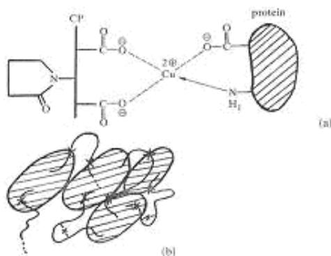
**Figure 103.** Schematic illustration of (a) the formation of chelate units between the functional groups of the copolymer (CP) and the protein antigen with participation of copper ions, and (b) the hypothetical structure of the triple polymer-metal complex of the protein antigen (crosses demote copper ions).
