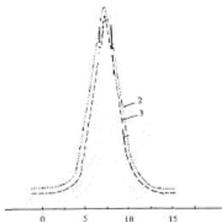
**Figure 89.** HPLC analysis of the soluble CPI-Cu<sup>2+</sup>-BSA mixtures were prepared at different conditions: (1) ternary mixture prepared in water; (2) ternary mixture prepared in 0.154 M NaCl; (3) CPI-Cu<sup>2+</sup>-BSA mixtures prepared in 0.154 M NaCl solution from the precipitate obtained after heating (37°C) the soluble ternary mixture in 0.154 M NaCl  $n_{Cu}/n_{AA} = 0.2$ ;  $n_{BSA}/n_{CP} = 1.0$ ; pH = 7.0.
