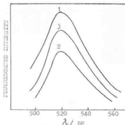
**Figure 122.** The fluorescence spectra of the model latex systems. 1-FITC-labelled latex ( $c=1,3 \cdot 10^{-8} \text{ cm}^{-3}$ ), 2- FITC-labelled latex + PVP-C<sub>2</sub>H<sub>5</sub> ( $10^{-6} \text{ M}$ ), 3- FITC-labeled latex + PVP-C<sub>2</sub>H<sub>5</sub> after adding of equal amount of nonlabelled latex ( $c=1,3 \cdot 10^{-8} \text{ cm}^{-3}$ ), pH=9. The turbidity spectra are subtracted
