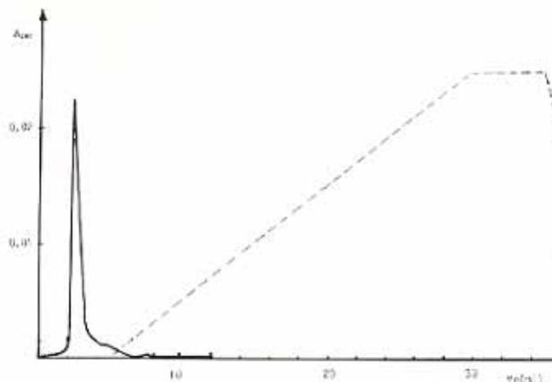
**Figure 101.** Anion-exchange chromatography of the matrix solution of the ternary mixture BSA-Cu<sup>2+</sup>-PAA. ( $C_{\text{PAA}} = 0.1$  g/dL);  $n_{\text{Cu}}/n_{\text{AA}} = 0.30$   $n_{\text{BSA}}/n_{\text{PAA}} = 1.0$ ; pH = 7; 25°C. Broken line corresponds to (NaCl) concentration gradient.
