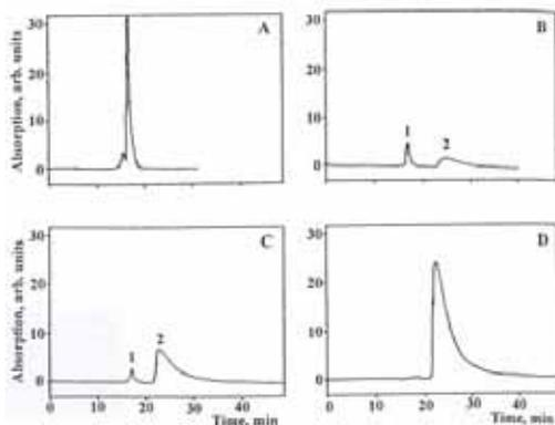
**Figure 93.** Gel filtration HPLC chromatograms of BSA (A) and of its mixtures with  $\text{Cu}^{2+}$  at different ratios of  $\text{Cu}^{2+}$  ions to BSA molecules ( $n_{Cu}/n_{BSA}$ ): 4 (B); 8 (C); 40 (D).
