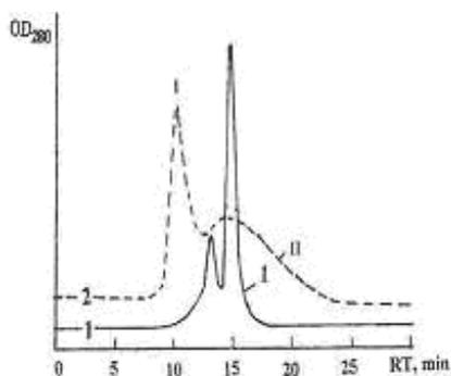
**Figure 168.** HPLC analysis of the solutions of pure BSA (1) and the product obtained from the BSA+betulin+carbodiimide mixture (2) prepared in phosphate buffer (pH 7); Uv – 280nm; 0.7mg/mL; 40g/Lc 1mL/min
