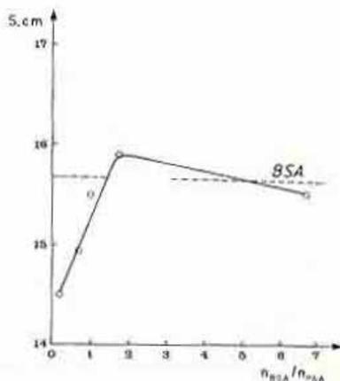
**Figure 104.** Dependence of the electrophoretic mobilities (distance-S) of the products of solution of the ternary mixture BSA- $\text{Cu}^{2+}$ -PAA on  $n_{BSA}/n_{PAA}$ ;  $C_{PAA} = 0.1$  g/dL  $n_{Cu}/n_{PAA} = 0.25$ ; pH = 7; 25°C. Broken line represents free BSA.
