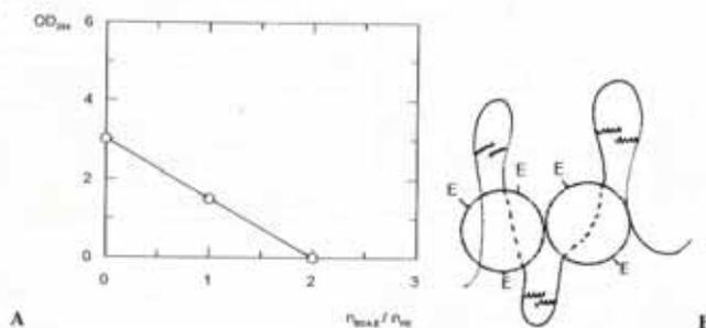
**Figure 152.** (a) Dependence of values of optical density ( $OD_{254}$ ) of matrix solution of mixture PVP ( $R_2.R_{16}$ )-BSA.E obtained by UV spectrophotometric analysis at 254 nm on  $n_{BSA}/n_{PE}$ - (b) A schematic presentation of the structure of BSA.E complexes with PVP ( $R_2.R_{16}$ ). For explanations see text
