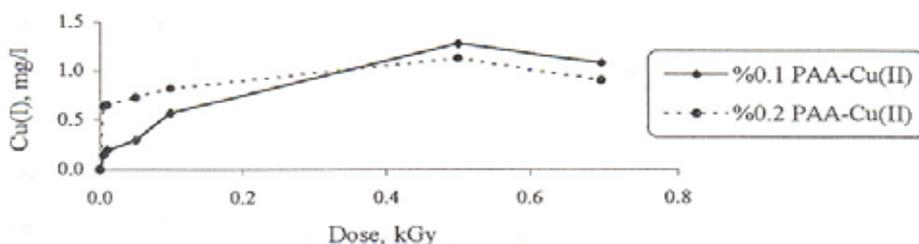
**Figure 191.** Effect of radiation dose on formation of Cu (I) in PAA-Cu(II) system; [Cu<sup>2+</sup>] = 1.388 x 10<sup>-3</sup> M, [PAA] = 0.1 g/dl and 0.2 g/dl,  $n_{\text{Cu}^{2+}}/n_{\text{PAA}} = 0.05$
