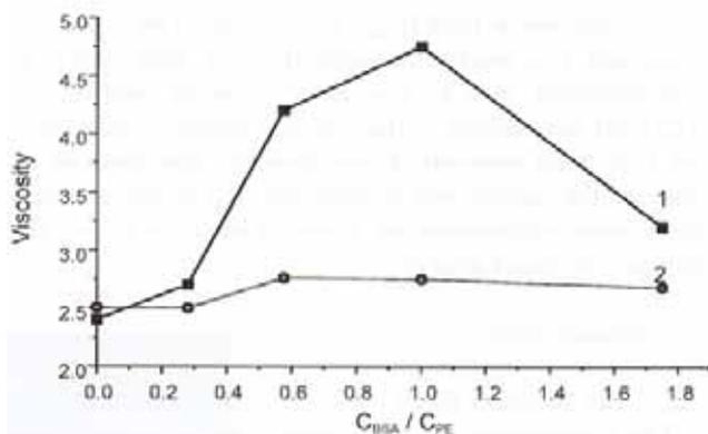
**Figure 107.** Dependence of viscosity ( $\eta_{sp}/C$ , dl/g) of reaction products (CP-EDC-BSA) (1) and mixtures (CP-BSA) (2) on the initial ratio BSA/CP in neutral water solution (PBS, pH 7). Molar ratio of  $[EDC]/[AA] = 1:2$ ; different BSA concentration; 23°C.
