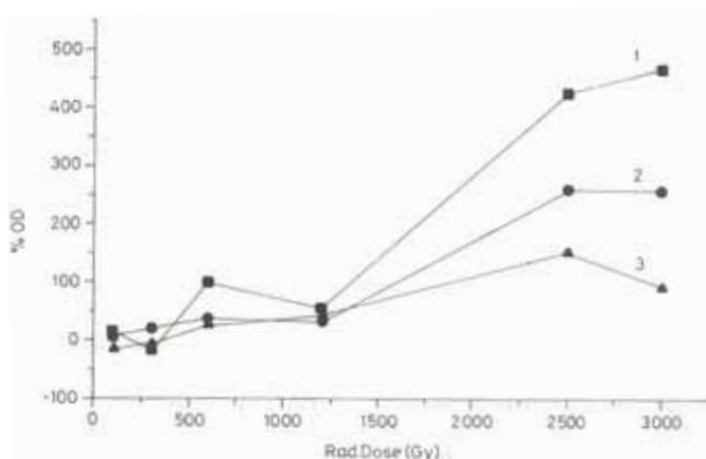
**Figure 188.** Percentage changes in optical density values %OD [ $\%OD = (\Delta OD / OD) \times 100$ ] %OD versus radiation dose (Gy). 1 – PAA; 2 - (PAA - SOD); 3 - SOD;  $C_{BSA} = C_{PAA} = 0.01$  g/l
