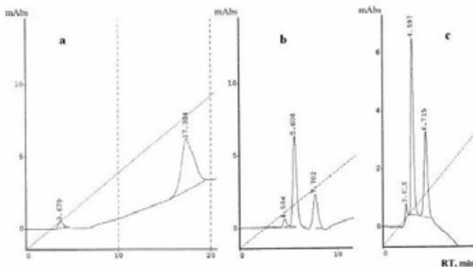
**Figure 177.** Ion-exchange HPLC results of BSA-CDI-Peptide mixtures
