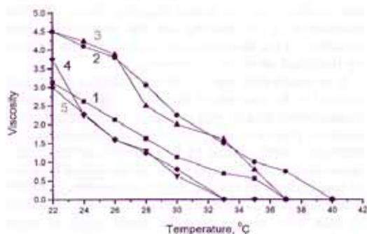
**Figure 12.** Dependence of viscosity (sp/c, dl/l) of solution of pure CP (1) and conjugates on temperature, preparing at different ratios: 0.28 (2); 0.59 (3); 1.14 (4); 1.70 (5)  $C_{cp} = 0.25$  l/dl, different protein concentrations. Phosphate
