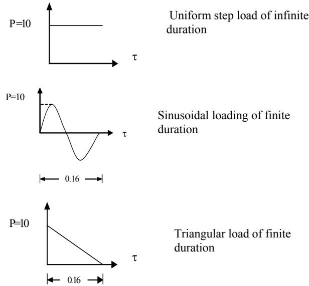
Figure 2. Dynamic loads considered in numerical applications
