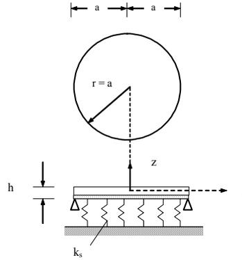
**Figure 1.** A schematic diagram of a circular plate on an elastic foundation
