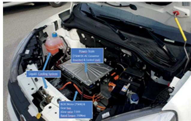
**Figure 29.** 75 kW liquid-cooled, fully-controlled three-phase DC-AC converter and control system on platform (car).
