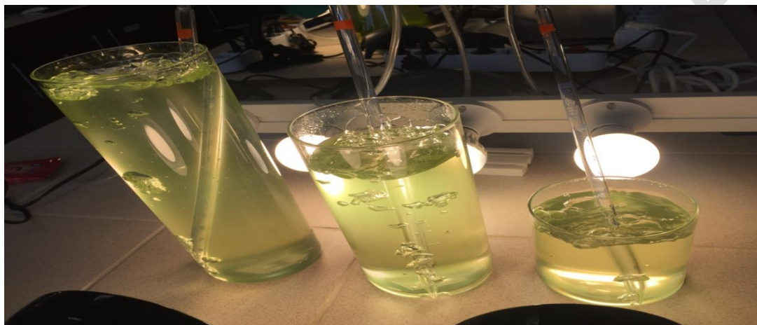
Figure 1. The photobioreactors with different height/diameter ratio
