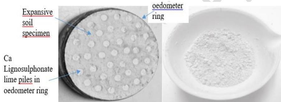
**Figure 2.** Ca Lignosulphonate lime pile (LLP) (left) in oedometer ring and CaLS lime mixture (right)
