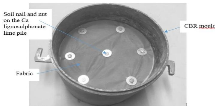
**Figure 8.** USIT specimen in CBR mold prepared for CBR swell test
