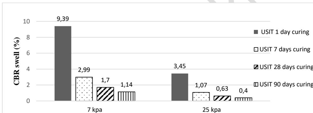
**Figure 9.** CBR swell values of USIT specimens
