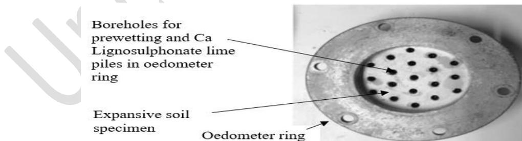
Figure 4. Number of piles in oedometer ring for USIT technique
