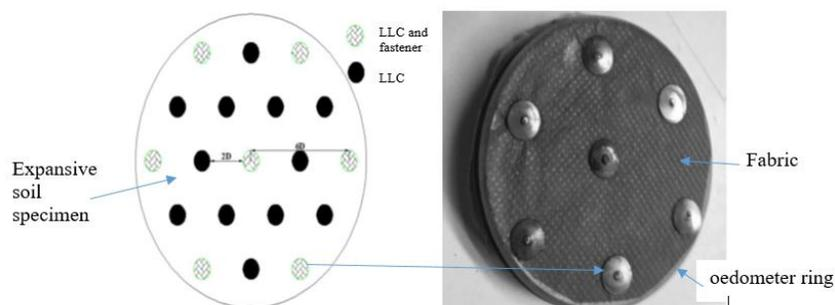
**Figure 6.** The plan of fasteners and final top view of the USIT specimen in oedometer ring
