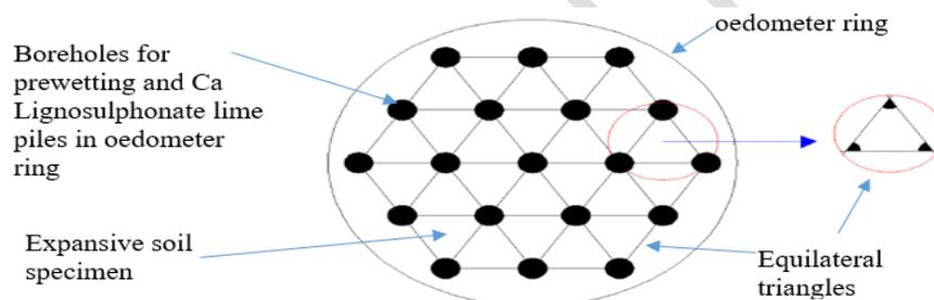
**Figure 5.** Equilateral triangles into the expansive soil specimen in oedometer ring
