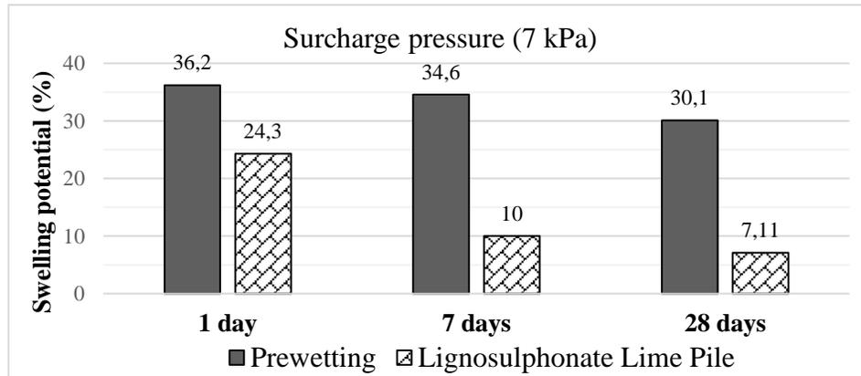
Figure 3. Swelling potentials of treated specimens with either prewetting or LLP
