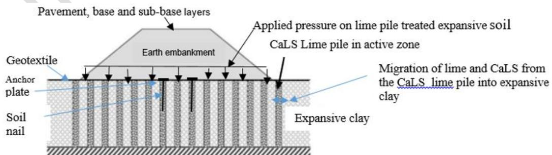
**Figure 1.** Unified Soil Improvement Technique under the pavement and embankment load
