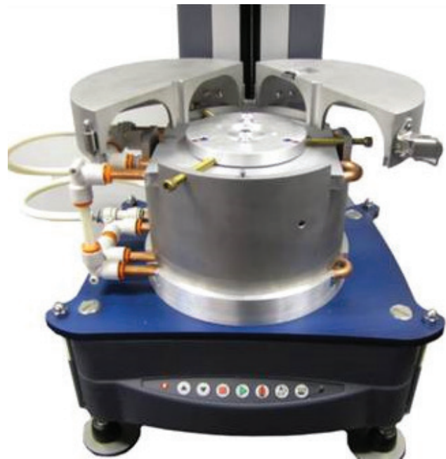
Figure 5. Rheometer to measure shear strength of MR fluids.
