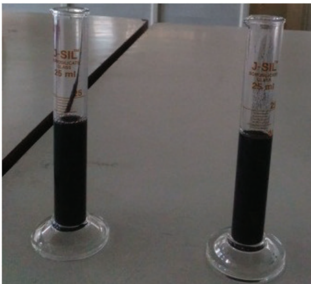
Figure 4. Glass jars to measure sedimentation in MR.
