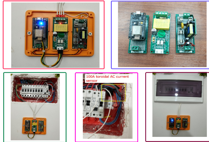
Figure 12. Installing AC smart plug in a real house. Measure the energy and analyze the consumption behavior
