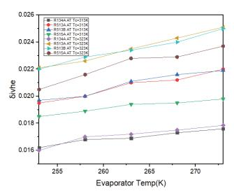
**Figure 11.** Efficiency defect of Internal vapour heat exchanger with Evaporator temperature.
