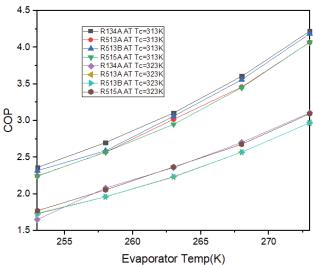
Figure 5. COP vs Evaporator temperature.
