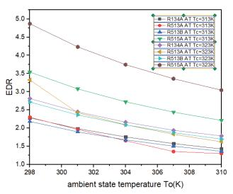
Figure 14. EDR vs Ambient state temperature (at  $T_E = 273$ K).
