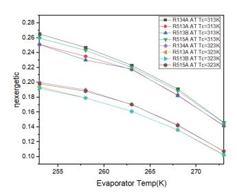
Figure 6. Exergetic efficiency vs Evaporator temperature.
