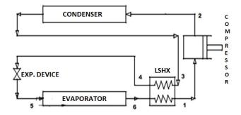
Figure 1. Refrigerator with LSHX.
