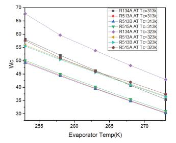
**Figure 3.** Compressor power consumption vs Evaporator temperature.
