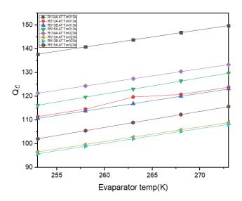
Figure 4. Cooling capacity Vs Evaporator temperature.
