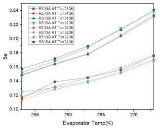
Figure 9. Efficiency defect of evaporator vs Evaporator temperature.
