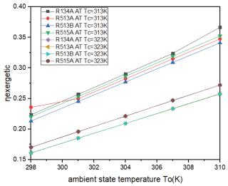
Figure 13. Exergetic efficiency vs Ambient state temperature.
