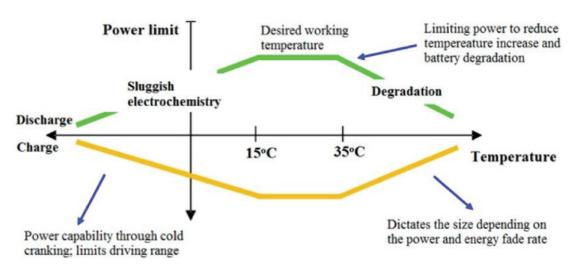
Figure 11. Working temperature interval of batteries [85].
