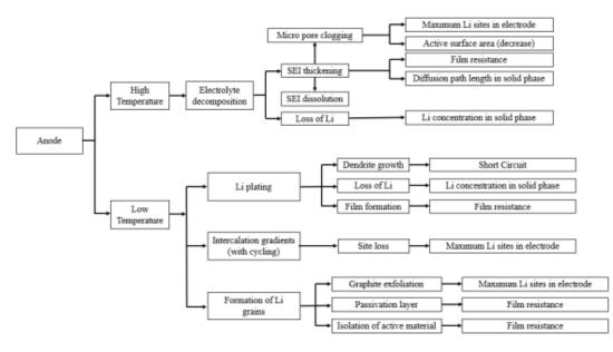
Figure 7. Negative electrode and temperature effect [43].
