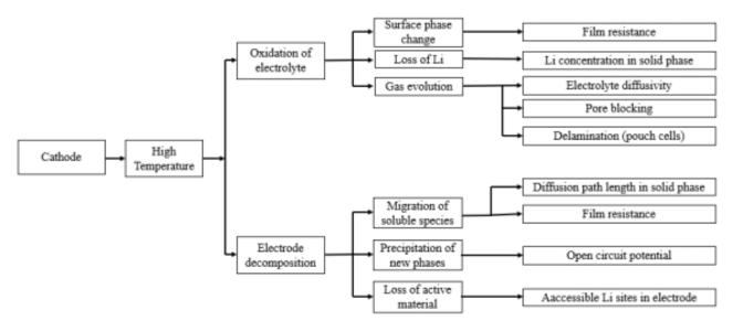
Figure 8. Positive electrode and temperature effect [43].
