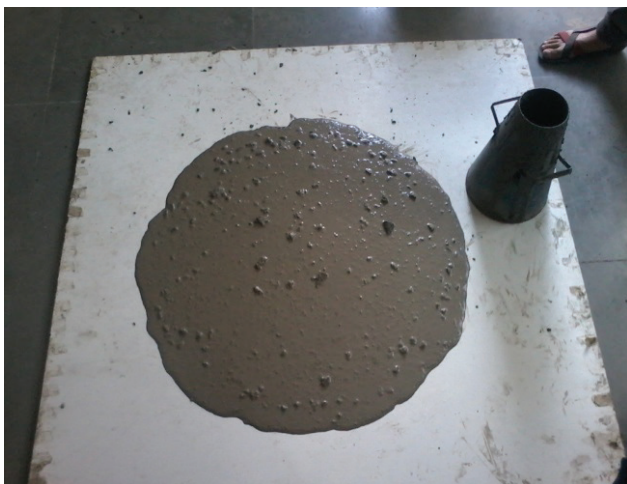
Figure 3. Slump flow of concrete.
