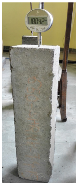
Figure 1. Shrinkage test setup
