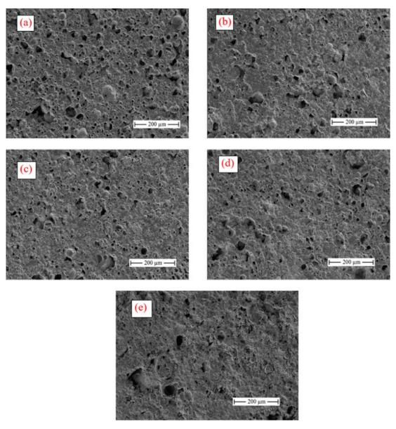
Figure 5. SEM analyses of sintered porous geopolymers MW0 (a), MW5 (b), MW10 (c), MW20 (d), MW40 (e).
