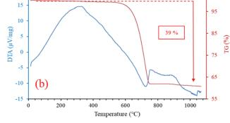
Figure 2. DTA/TG analysis of Tunçbilek FA (a) MW (b).
