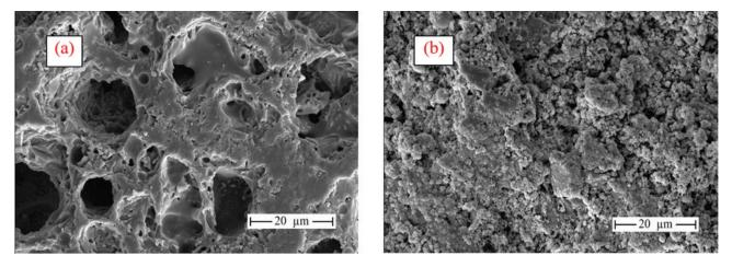
**Figure 6.** SEM analyses of sintered porous geopolymers; MW0 (a), MW40 (b).
