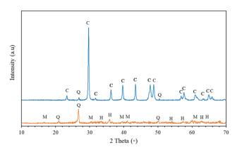
**Figure 1.** XRD spectrum of Tunçbilek FA (a) and MW (b). (C: calcite, Q: Quartz, M: Mullite, H: Hematite)
