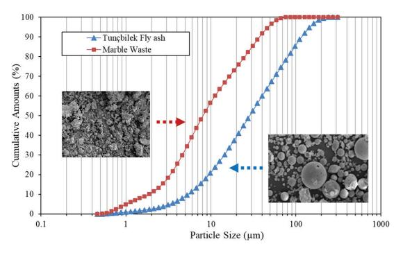
Figure 3. Particle size distribution of Tunçbilek FA and MW.
