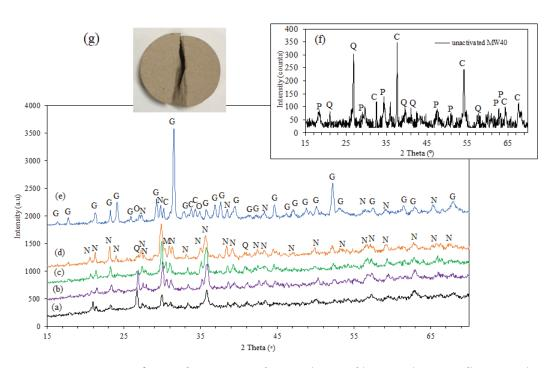
**Figure 8.** XRD spectra of sintered porous geopolymers; a) MW0, b) MW5, c) MW10, d) MW20, e) MW40, f) un activated MW40, g) un activated MW40 photograph (G: Gehlenite, N: Nepheline, Q: Quartz, O: Orthoclase, C: Calcium Iron Oxide, P: Portlantide (Ca(OH)2)).
