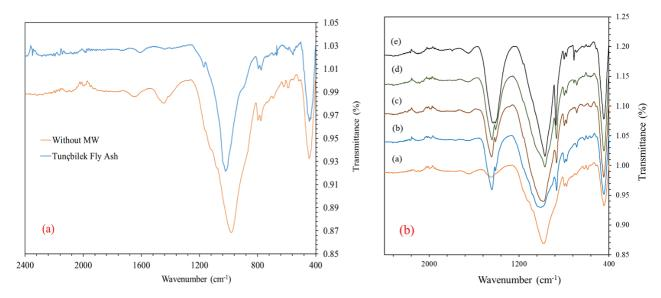
**Figure 4.** FTIR spectra of raw Tunçbilek FA and MW0 geopolymer (a) and geopolymers MW0 (a), MW5 (b), MW10 (c), MW20 (d), and MW40 (e) (b).
