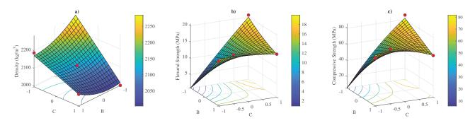
Figure 7. a) density b) flexural c) compressive strength regarding B and C while constant A component.
