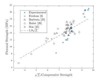
**Figure 3.** Flexural and compressive strength relationship with literature.
