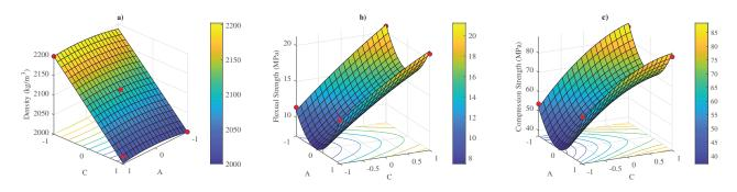
Figure 8. a) density b) flexural c) compressive strength regarding A and C while constant B component.
