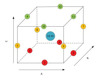
Figure 1. Experimental points according to Box-Behnken RSM.
