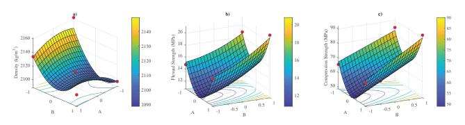
Figure 9. a) density b) flexural c) compressive strength regarding B and C while constant A component.
