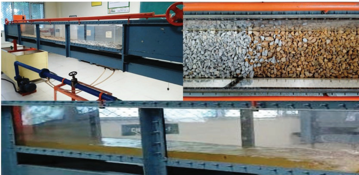
Figure 3. Arrangement of gravel bed materials and the formation of hydraulic jumps in the channel.
