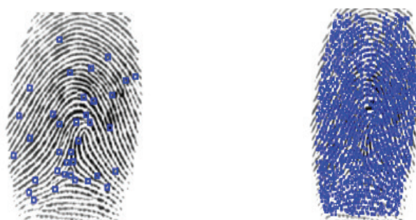
Figure 10. Extraction of minutiae and SIFT feature points from a single image. First image shows 36 Minutia points second image shows SIFT feature points.
