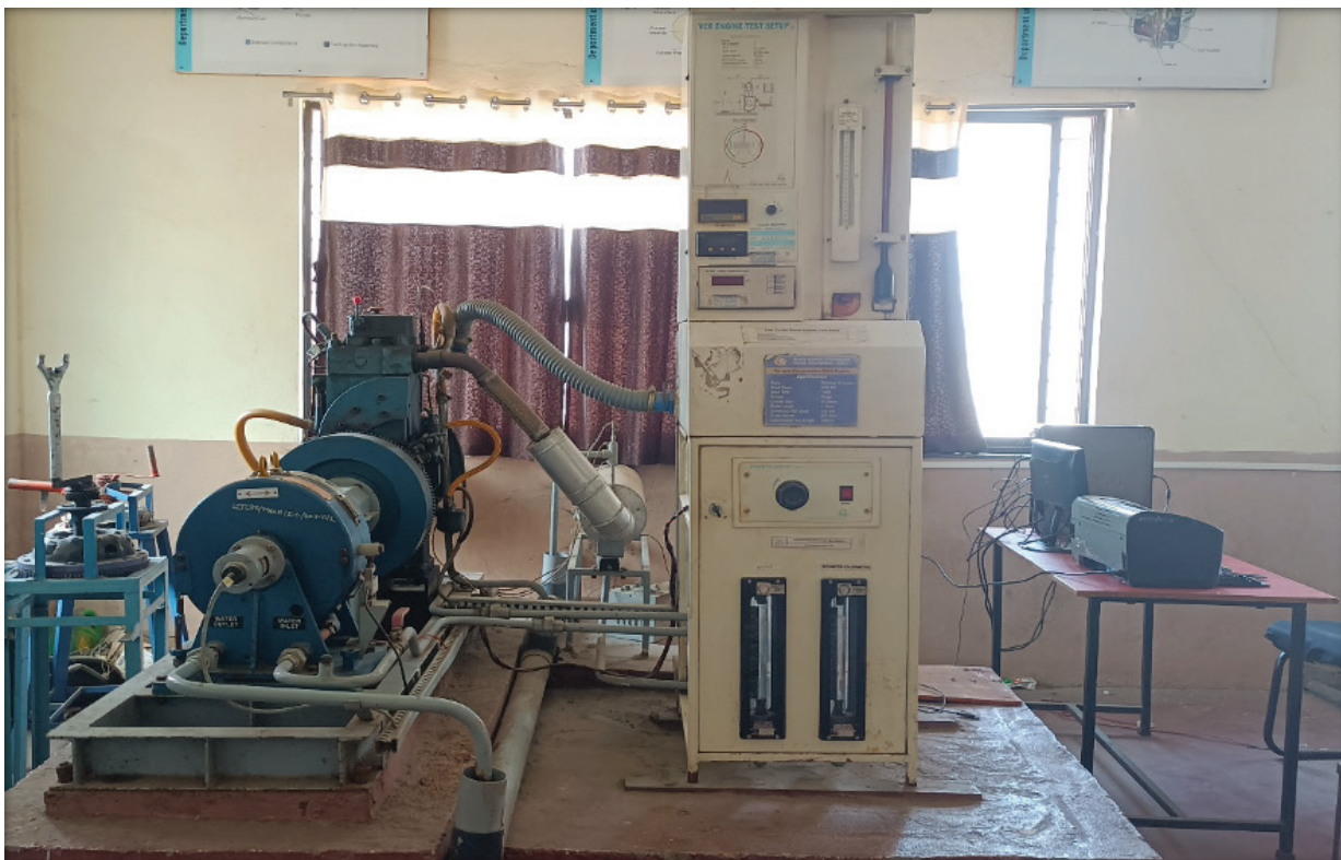
Figure 3. Experimental set-up of four stroke single cylinder engine.
