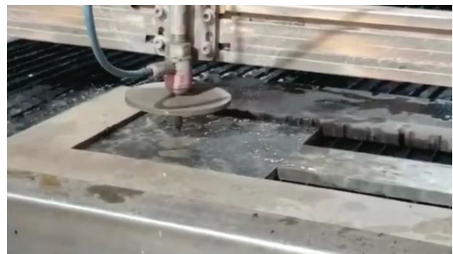
Figure 1. Setup for AWJM operations.
