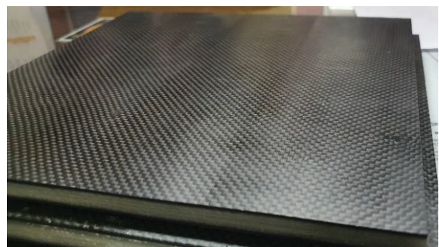
Figure 2. Coremat based CFRP sheet.
