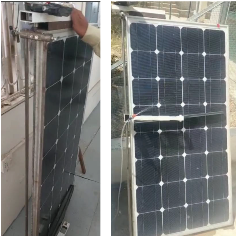
Figure 6. Photograph of the wiper-based cleaning solution installed and operated on 120 W solar panel. Cleaning time is under 7 minutes.
