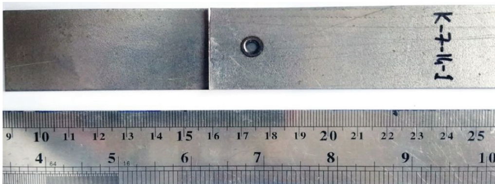
Figure 1. The overlapped RSW joint (EN ISO 14273 standards - tensile shear and Fatigue test).
